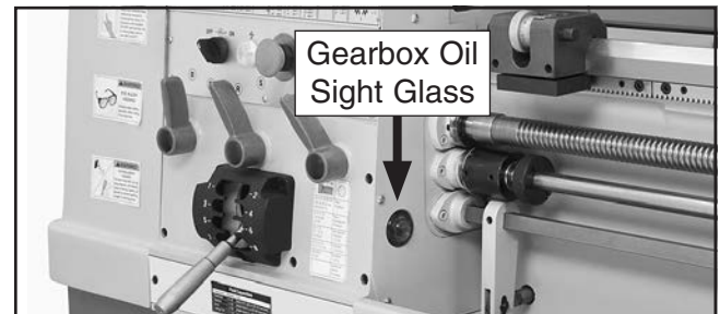
Figure 101. Location of gearbox oil sight glass.
